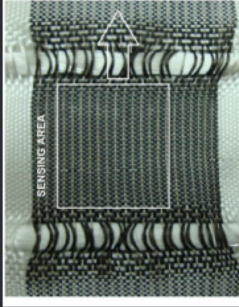
Figure 3. Configuration of the 3D flexible piezoelectric sensor fabric. The sensing area is highlighted in the white color; the silver spacer parts are black. The sensor structure in clear area is highlighted on the right hand side. [50] (note, which is available at www.scribd.com/doc/100000000/3D-flexible-piezoelectric-sensor-fabric )
