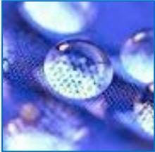
Superhydrophobic nanocoating (lotus effect)
